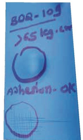
maintains batch record of scratch & impact tests on powder coated panels
