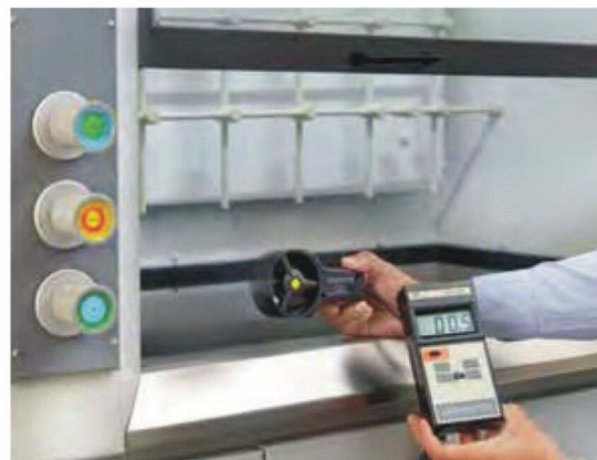
Required average face velocity 0.5 m/s
